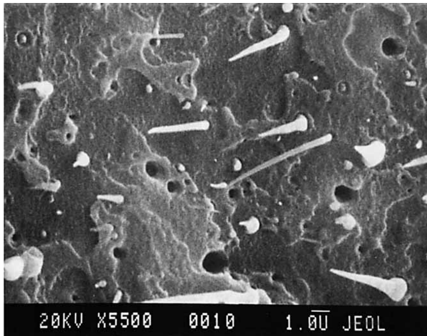
Figure 12 Fiber cross section of an as-spun 20% Triad2 (2 : 6 : 7) blend fiber.
